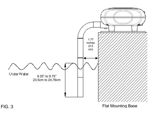
WARNING: The pool alarm may not function properly if your pool's water level is not maintained and the bottom of the tube is not between 9.25 inches (23.5 cm) and 9.75 inches (24.76 cm) below the water line.
